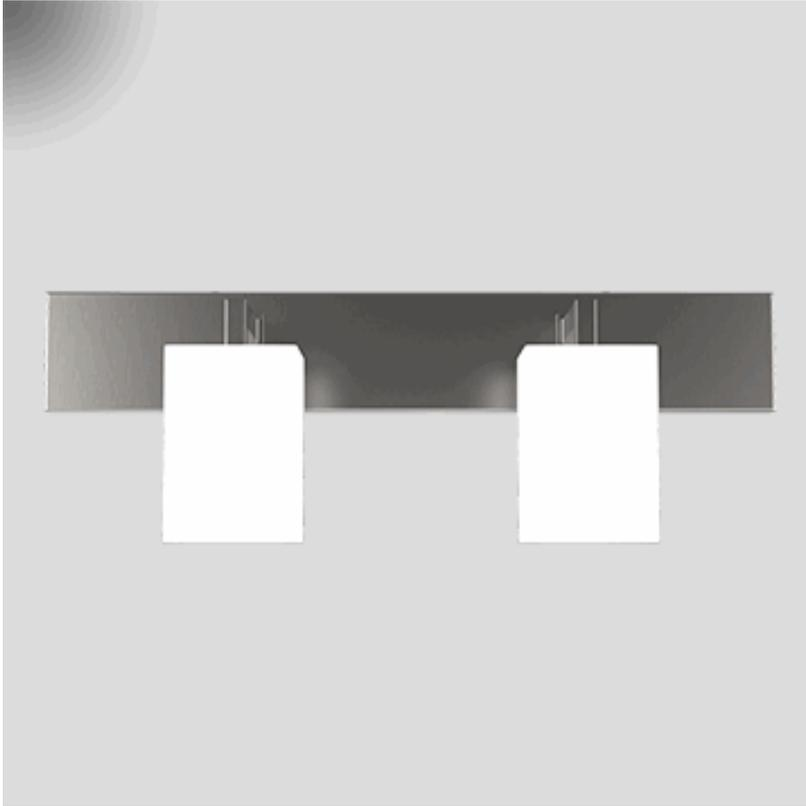
24" Brushed Nickel Vanity Fixture, 8.5" High, two medium base sockets, direct wired, with Frosted White Glass Diffusers. Recommended two 1100 lumen LED bulbs.
